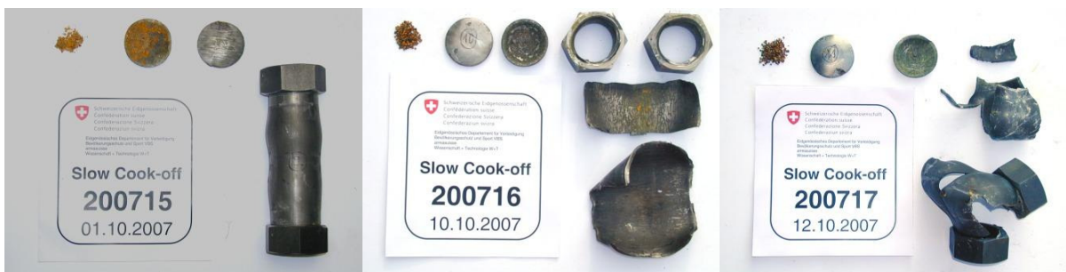
Fig. 2 Cook-off steel tubes after the experiments carried out with three temperature modes described above. From left to right: temperature ramp 3.3 K/h, temperature ramp 1.0 K/h and heat-wait-search mode.
