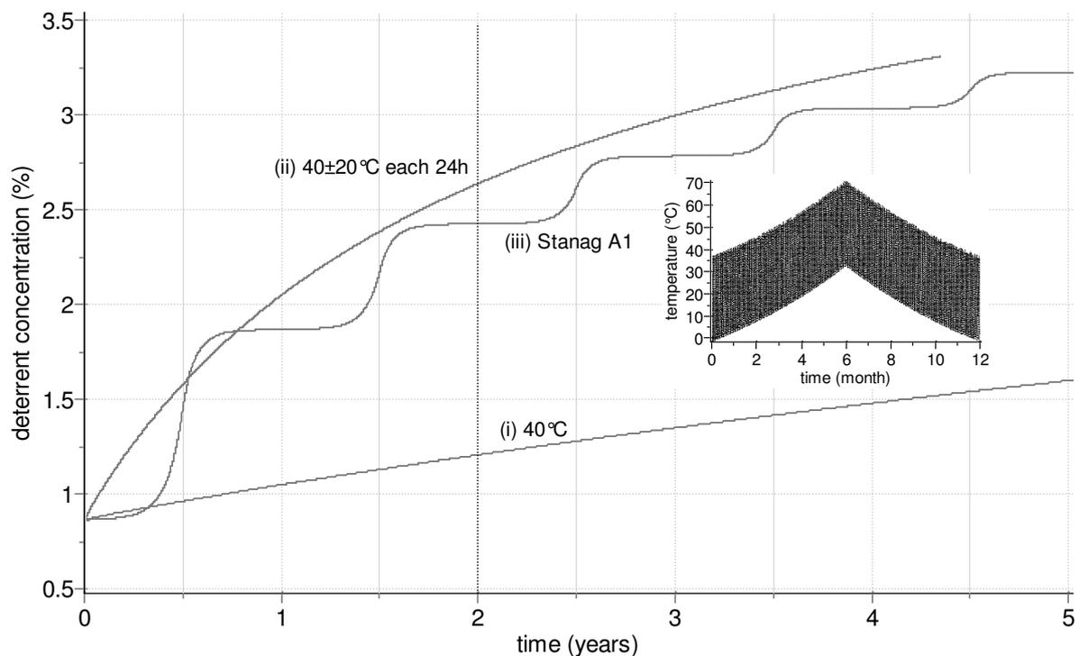
**Fig. 6** Average concentration of detergent in zone II (see Fig.5) in double base propellant as a function of aging time under isothermal ( $40^{\circ}\text{C}$ ), oscillatory ( $40^{\circ}\text{C}\pm 20^{\circ}\text{C}$ , 24 h period) temperature conditions and high climatic category A1 according to STANAG 2895. The storage/transit temperatures recorded during one year in the climatic category A1 are presented in the inset.
