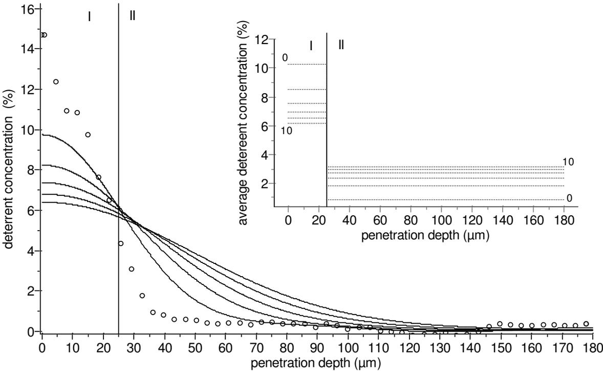
**Fig. 5** Initial experimental (symbols, data source: Royal Military Academy, Bruxelles, Belgium) and simulated (lines) concentration distribution of deterrent (DBP) in a double base ball powder propellant during an accelerated aging at 80°C. Aging times in the range of 0-10 days are marked on curves. The average concentrations of deterrent in zones (I) and (II) after aging time between 0 and 10 days are displayed in the inset.
